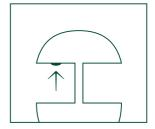
To temporarily turn off the light, press the button under the light unit. It will stay off until its set wake up time. Press again to turn the light back on.
