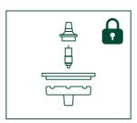
Make sure that the preassembled center part **(P3, P4, P5 and P6)** is firmly locked. Then place into the water bowl.
