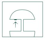
Set the sleep timer by holding the button under the light unit for 3 s. Lights will blink 2 times and then turn off.
