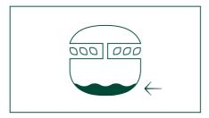
If the pump starts being noisy the water level is too low. You can check the water level by lifting up the center part **(P3, P4, P5 and P6)**. When the water has run out the light will start flashing.
